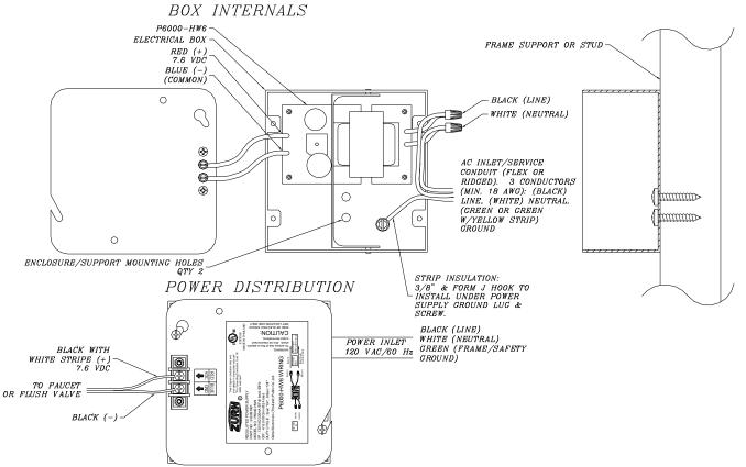
Internal conductor terminations/connections shall be implemented using UL approved screw terminals, wire nuts, insulated/isolated crimp splices, or soldered using hook & loop method with the solder joint(s) post insulated or as specified within the National Electrical Code (NEC) and/or superseding relevant local specified code(s).
